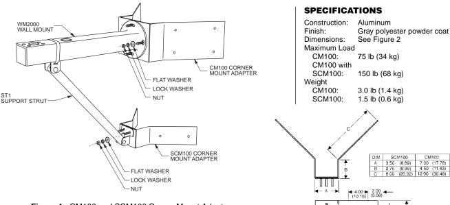
Figure 1. CM100 and SCM100 Corner Mount Adapters
